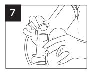
The tubing should still be **CONNECTED** to the adapter cap(s) and tubing adapter. If you have taken these apart, attach tubing to adapter cap(s) and the tubing to the tubing adapter.
